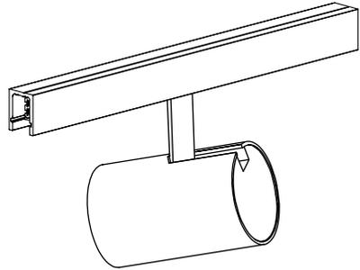
**Standard Mounting** - CT1 track head features a tilt-lock screw that utilizes a 1/16" Allen wrench for tightening and loosening, tighten once aiming is completed. CT2 features tool-less tilt-lock.
