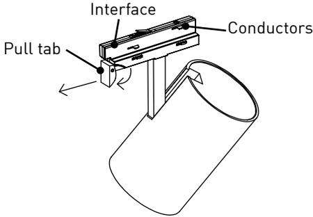
Align interface with track and gently push track head adaptor into track section by applying even pressure to interface until seated. Slide locking tab back to lock into place. Reverse process to remove track heads by sliding locking tab open and pulling straight down on interface.
