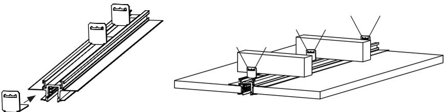
Recommend pinning top of track to framing to ensure track is level.
