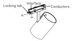
With conductors retracted and track head in a tilted position, align conductors with busbar and gently push track head adaptor into track section by applying even pressure to interface until both conductors engage busbar. Slide locking tab back into place. Reverse process to remove track heads by sliding locking tab open and pulling straight down on interface.
