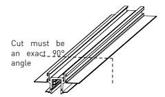
Ensure rotation of saw blade is directed towards busbar.
