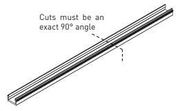
Cut a 1.25" notch into the end of the track gap cover that will be installed over the dead end fitting.
