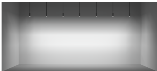
10FT CEILING 36" SETBACK / 48" ON CENTER SPACING
