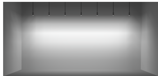
12FT CEILING 36" SETBACK / 48" ON CENTER SPACING
