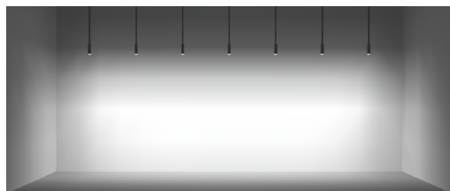
8FT CEILING 36" SETBACK / 48" ON CENTER SPACING
