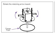
Raise retaining cartridge into the housing, rotate retaining arms outward, and tighten retaining screws until the bottom of the cartridge is flush with the ceiling plane. Raise canopy plate.
