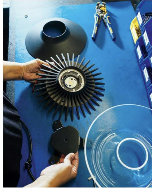
A light being assembled at Lucifer's factory. Photograph by Josh Huskin
