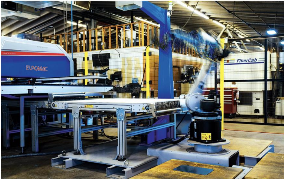
A turret punch in motion at Lucifer Lighting.
