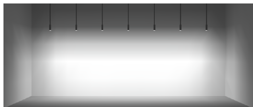
8FT CEILING 36" SETBACK / 48" ON CENTER SPACING
