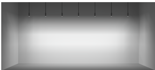
10FT CEILING 36" SETBACK / 48" ON CENTER SPACING
